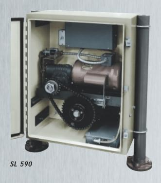
The SL 590 is designed for heavy-duty industrial applications where the gate is up to 90 feet long weighing as much as 2500 pounds and handling up to 25 cycles per hour. This gate operator has been built to deliver years of dependable performance by utilizing a high starting torque motor, with built-in overload protection, driven limit switches and a solenoid activated brake. This configuration reduces wear and tear on the operator as well as the gate.
