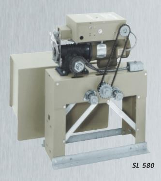
The SL 580 is an electric slide operator designed for heavy-duty commercial and industrial applications where the gate is up to 80 feet long weighing as much as 1900 pounds and handling up to 25 cycles per hour. This gate operator has been built to deliver years of dependable performance by utilizing a high starting torque motor with built-in overload protection, driven limit switches and a solenoid activated brake. This configuration reduces wear and tear on the operator as well as the gate.
