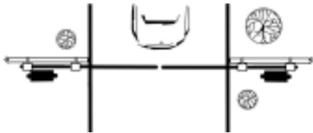
DOUBLE GATE WITH TWO UNITS
